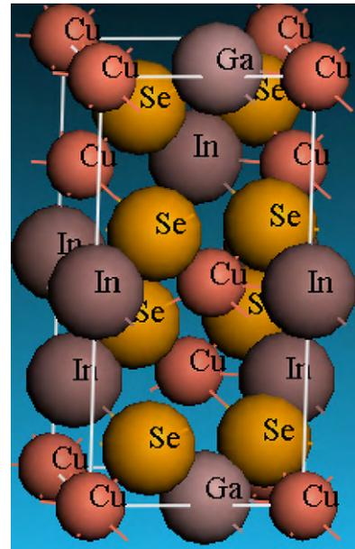
Fig. 3. Chalcopyrite structure of CuIn<sub>0.75</sub>Ga<sub>0.25</sub>Se<sub>2</sub>.
