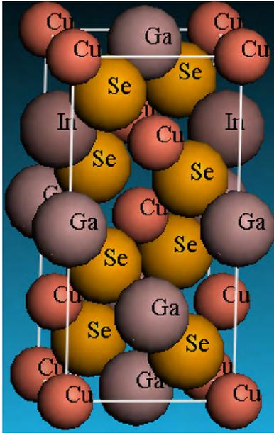
Fig. 1. Chalcopyrite structure of CuIn<sub>0.25</sub>Ga<sub>0.75</sub>Se<sub>2</sub>.
