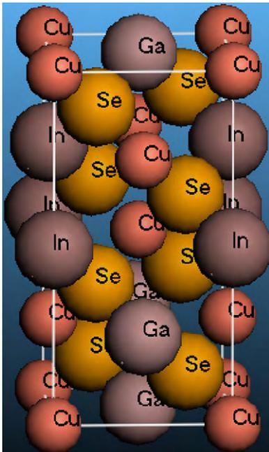
Fig. 2. Chalcopyrite structure of CuIn<sub>0.50</sub>Ga<sub>0.50</sub>Se<sub>2</sub>.
