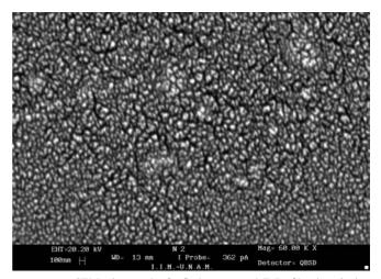
FIGURE 5 SEM micrograph of a flash-evaporated ZnPc film deposited at a substrate temperature of  $T_s = 373$  K
