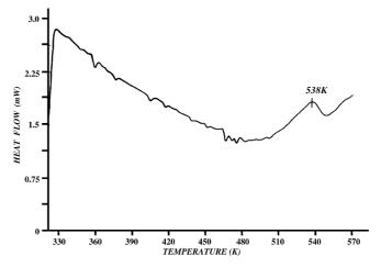
FIGURE 8 Phase-change curve for a typical flash-evaporated ZnPc thin film
