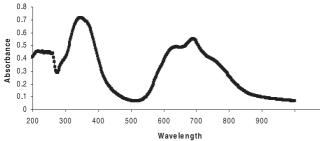
FIGURE 9 Absorption spectra for a typical flash-evaporated ZnPc thin film
