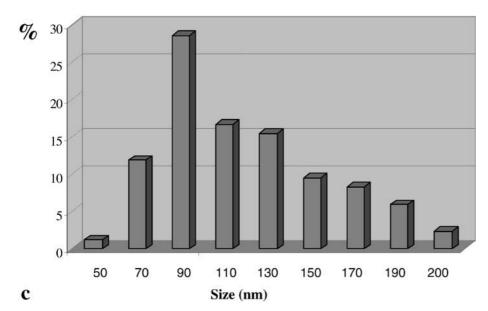
FIGURE 6 Three-dimensional SPM nanoscope analysis of the surface of flashevaporated ZnPc film deposited at a substrate temperature of  $T_s = 373$  K. **a** Threedimensional image, **b** sectional analysis indicating the size distribution and **c** sizedistribution plot
