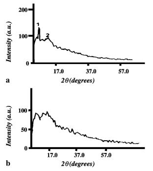
FIGURE 4 XRD pattern of the flash-evaporated ZnPc film at a substrate temperature of **a**  $T_s = 303$  K and **b**  $T_s = 373$  K
