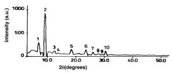
FIGURE 2 XRD pattern of the bulk ZnPc powder
