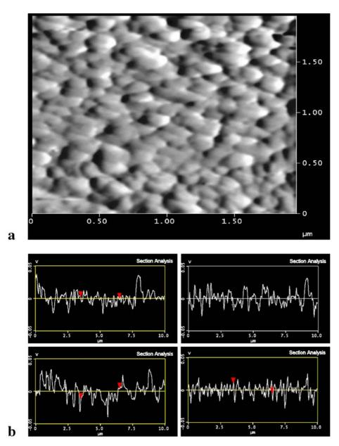
FIGURE 7 Surface analysis of the flashevaporated ZnPc films from the SPM nanoscope in deflection mode. **a** Deflection-mode image and **b** plot of potential developed at various sections related to composition and structural changes
