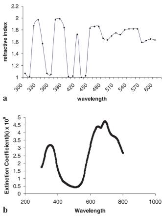
**FIGURE 11** Variation of **a** refractive index (n) and **b** extinction coefficient (k) with wavelength for a typical flash-evaporated ZnPc thin film
