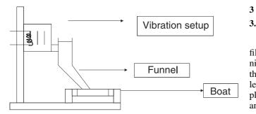
FIGURE 1 Flash-evaporation setup
