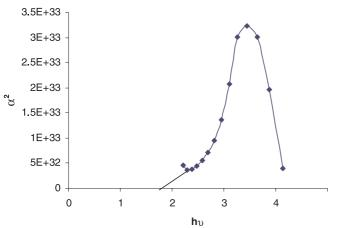
FIGURE 10  $\alpha^2$  versus photon-energy curve for a typical flash-evaporated ZnPc thin film
